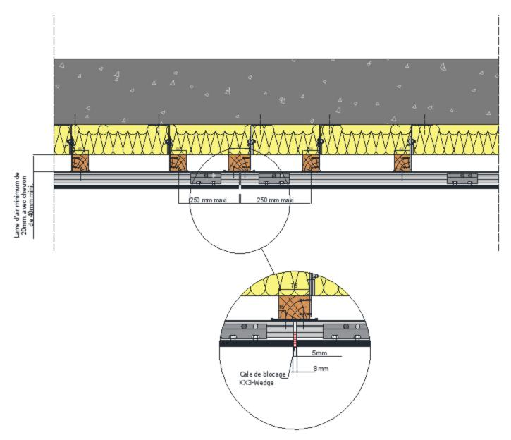
Figure 15 - Joint vertical (coupe horizontale)
