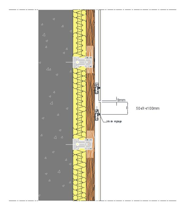
Figure 16 – Joint Horizontal (coupe verticale)
