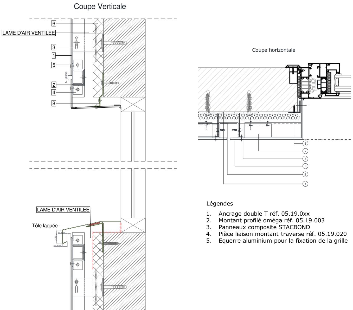
**Figure 11 – Encadrement de baie pose unidirectionnelle**
