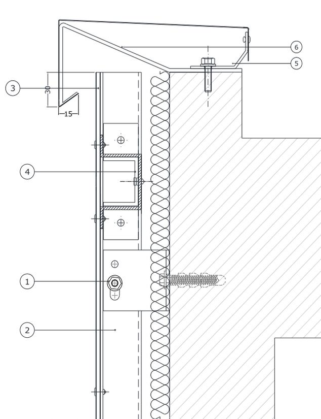
**Figure 7 – Départ de bardage**
